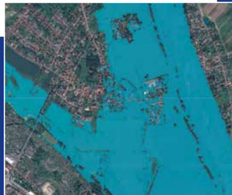
Detailed mapping of flooded urban areas using very high resolution optical data
